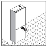
If after having carried out the previously described operation there is still some space left between the appliance and the kitchen unit, fit the trimming provided together with the appliance on the stop strip (A).
